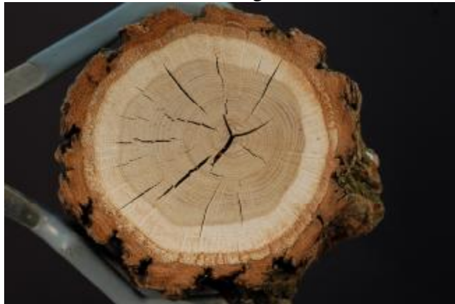
Fig.1. Note the checks and cracks in the end grain of this seasoned oak.
